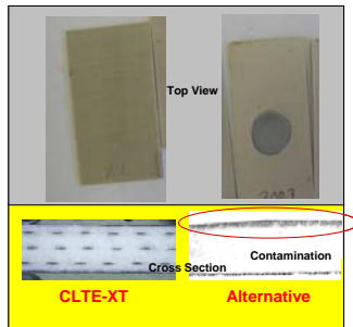
Figure 6. Exposure to Low Surface Tension Contaminant
