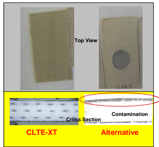
Figure 6. Exposure to Low Surface Tension Contaminant
