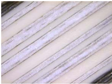
Fig. 8 20 Layer Board of CLTE-XT and SPEEDBOARD® C
