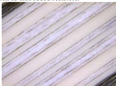
Fig. 5 20 Layer Board of CLTE-XT and SPEEDBOARD® C
